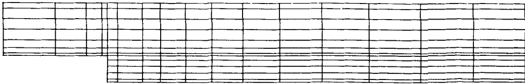
Figure 25. Finite element mesh for flow over a backward facing step: Number of elements = 172; Number of points = 201
