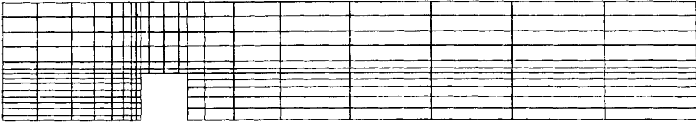
Figure 38. Finite element mesh (II) (extended version of mesh (I)): Total number of elements = 224; Total number of points = 264
